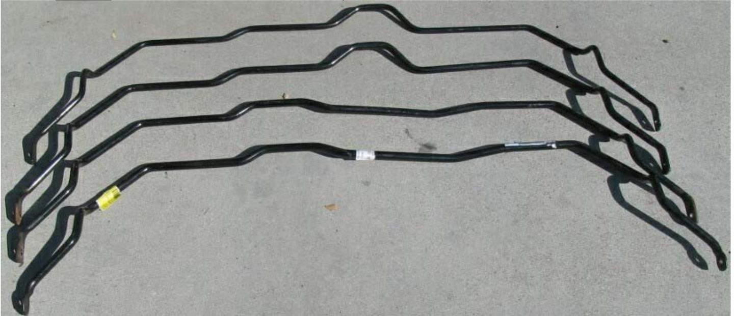
Early models, up to 9/92 had a loop that went around the front of the differential mount. From 9/92, the bar went between the differential and differential mount. Eliminating the “loop” increased stiffness.
