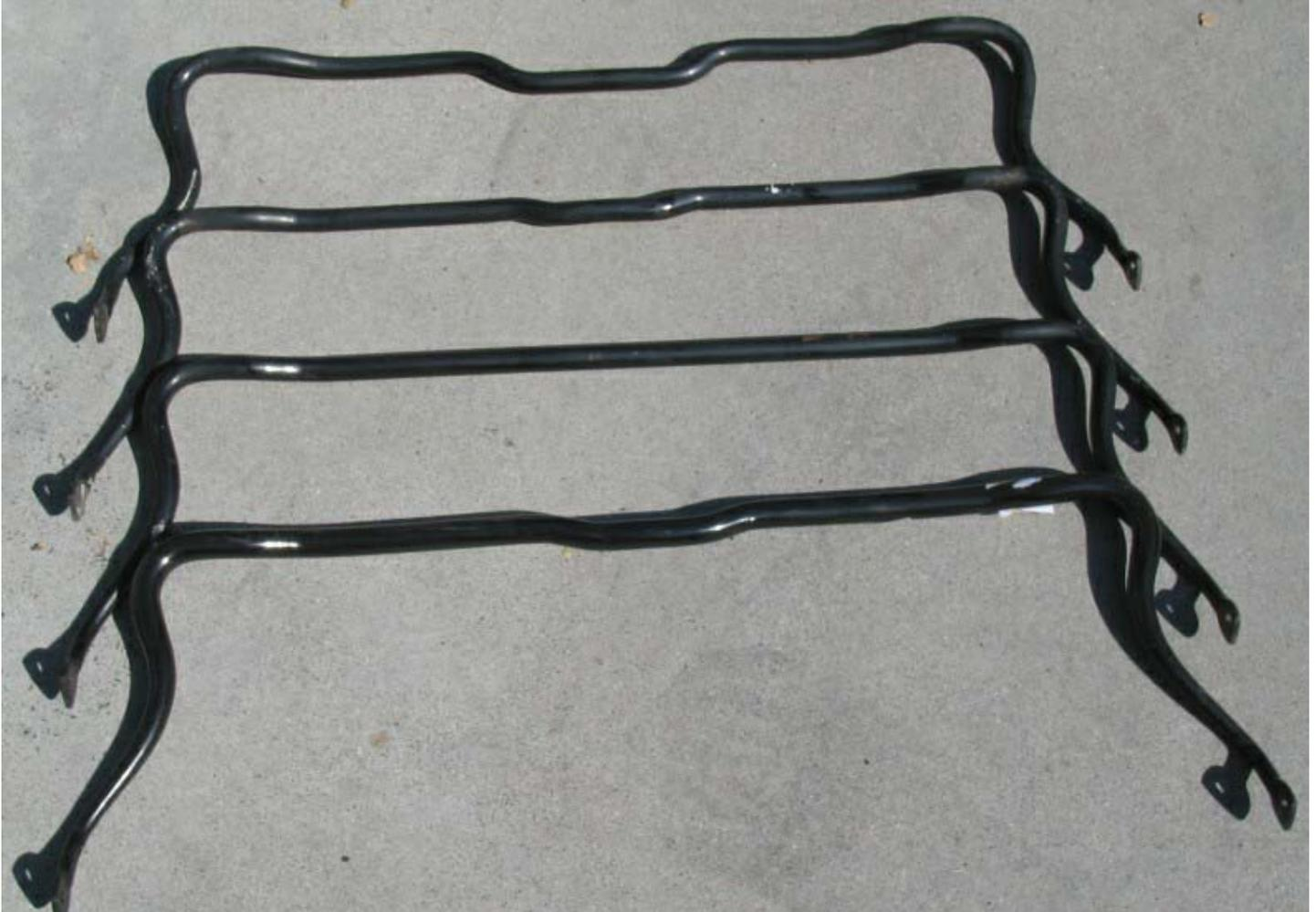
Part# 31 35 1 131 620 (far right) anti-sway bar arms are  $\frac{3}{4}$  inch longer as illustrated below and were used on subframes **without** the “X” frame stiffener that was introduced on models produced after 4/92,
