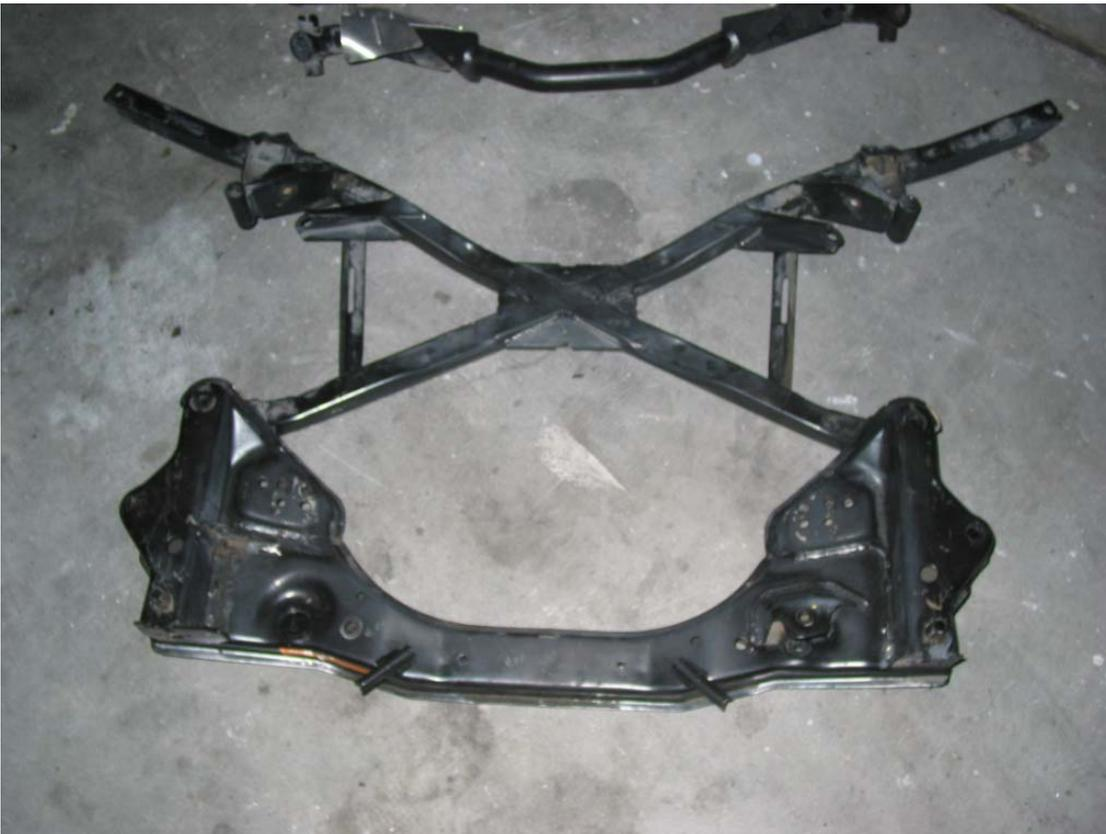
**Comparison of front anti-sway bar mounting position**
