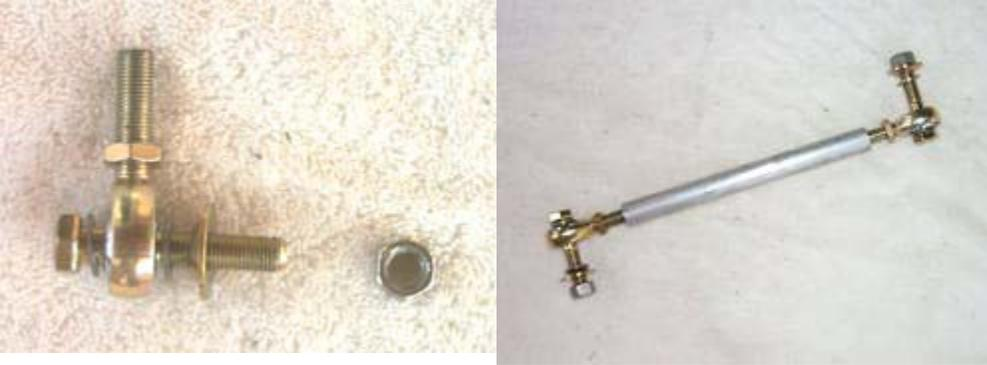
whole assembly with increase or decrease depending on the direction which you turn the rod. Tighten the jam nuts when the desired length is achieved.
