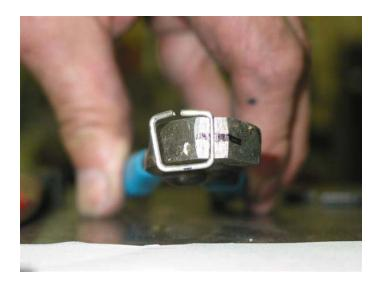
Now take the roll pin and insert one end of the bent wire into the open end of the roll pin.
