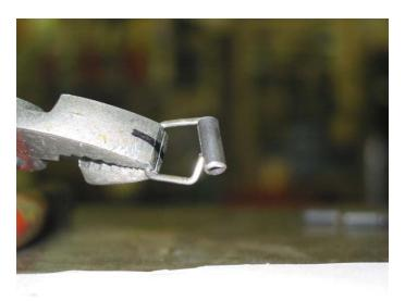
Spread the wire enough so that you can put the other end fo the wire into the opposite end of the roll pin.
