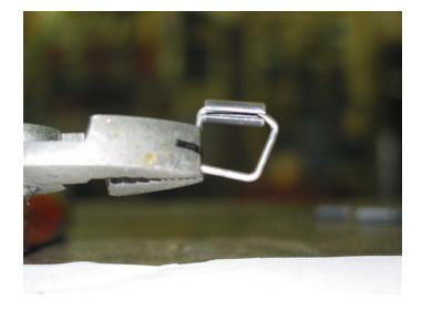
Gently squeeze the wire together at the roll pin to close the gap and make a good square shape, this may take a little effort depending on how much the wire was bent to get it into the roll pin. I have done hundreds of these and it is still challenging for me! But the results will be good!
