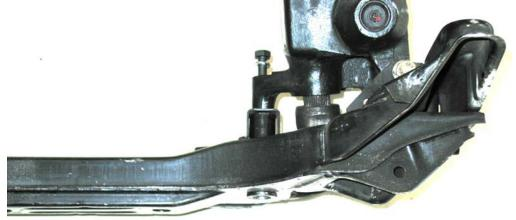
6. While maintaining the pressure on the dowel to keep it seated against the lower sub-frame material, weld around the flange of the dowel.
