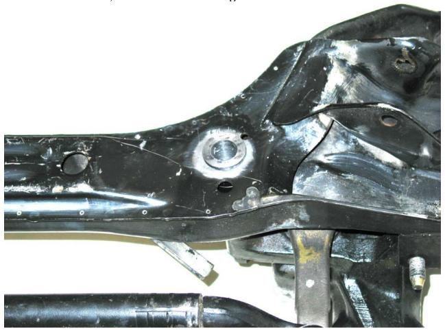
7. After welds cools, tighten bolt to attach the steering box securely to the dowel. I would recommend painting the area to prevent corrosion in the future.
