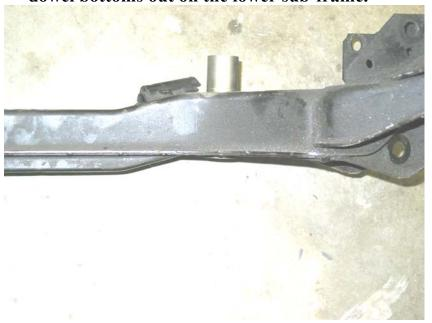
a. If the bracket has not broken, just feed the dowel thru the lower hole all the way to the bottom of the bracket and do not use the larger flat washer, use lock washer under the head of the bolt and tighten securely. The car may be driven and welding of the dowel to the lower sub-frame material may be done at anytime in the near future.
