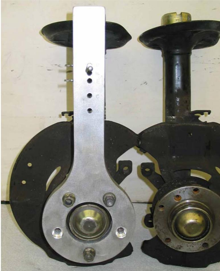
4. Loosen wing nut and feed measurement rod thru hole “G” of the tool until it just touches the strut. Make sure all dirt and contamination is off the strut in the measurement area. It is also suggested to measure the strut that was not subjected to damage first. Tighten the wing nut on the side of the gage to hold the measurement rod in place. **Do not over tighten wing nut, just snug up.**
