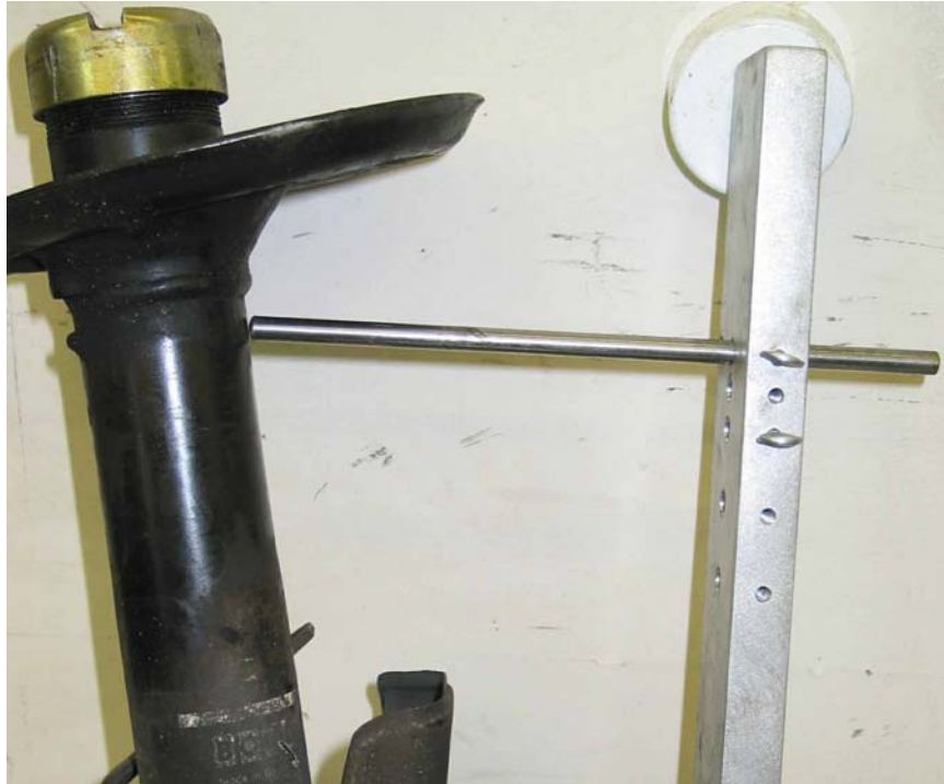
Picture #1 Measurement rod calibrated to damaged strut
