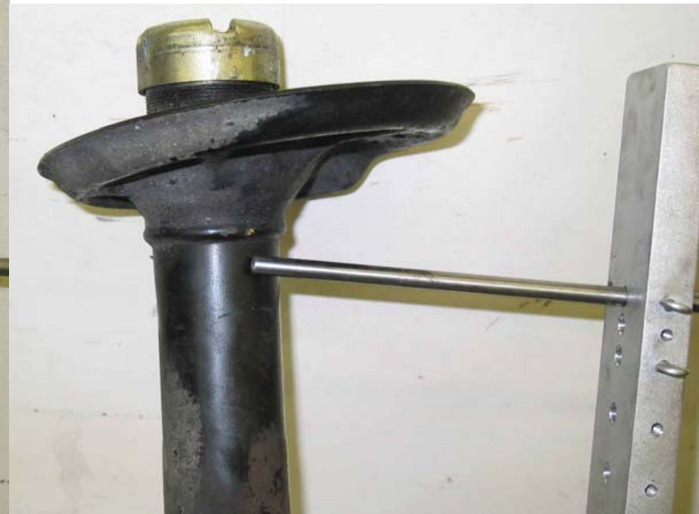
Picture #4 Top of the wheel inward (additional negative camber)
