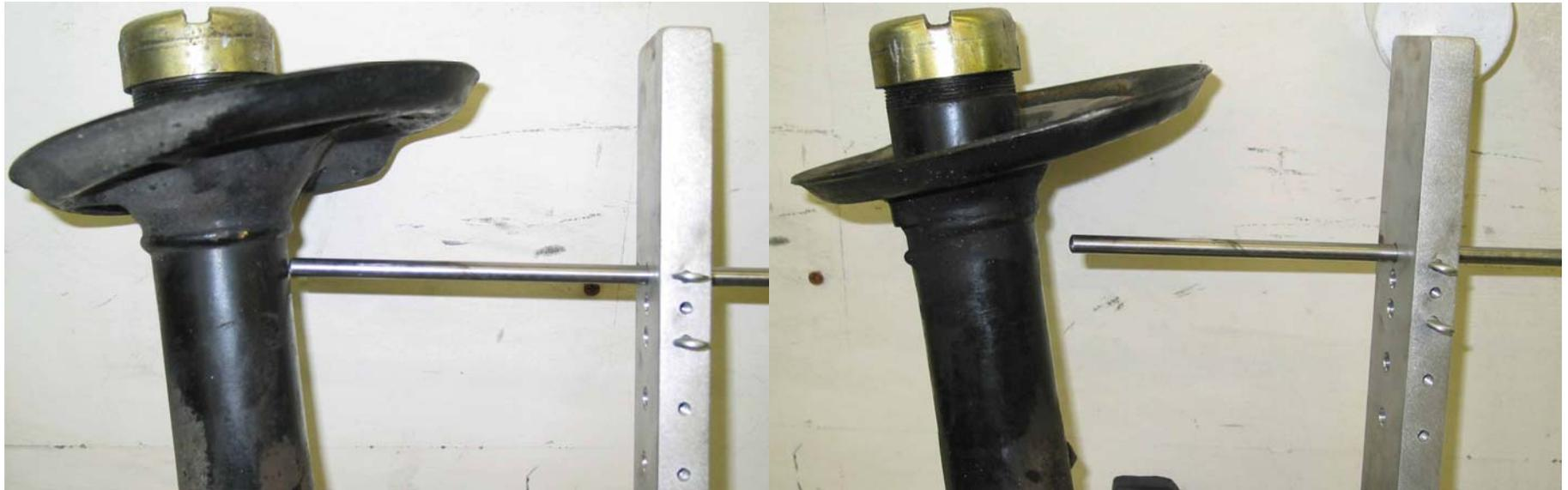
**Measurement rod set on good strut first**
