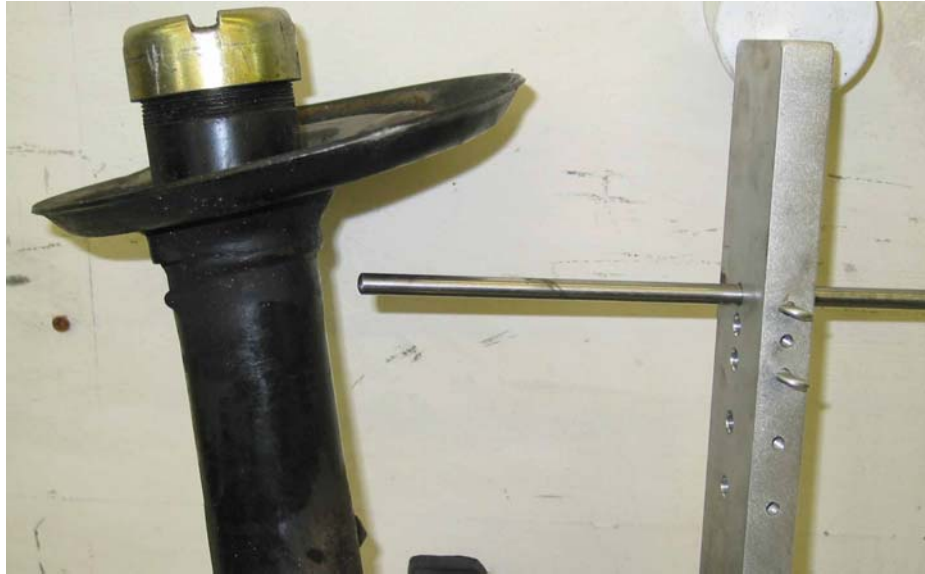
Picture #3 Top of the wheel outward (additional positive camber)
