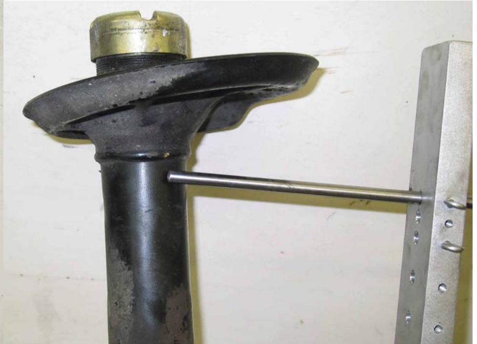
Picture #2 Measurement rod will not clear the strut and difference will be hard to measure
