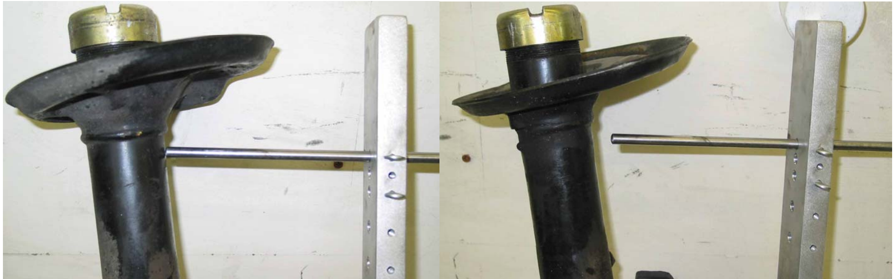
Measurement rod set on good strut first
