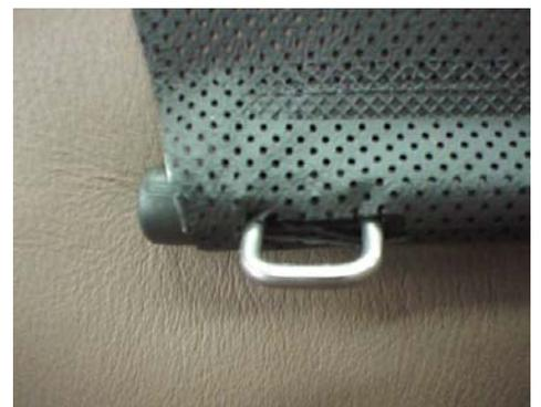
**You are finished! Do not drive with rear windows open and the sunshade out, you will destroy the headliner hooks and these have no replacement yet, I'm working on it!**
